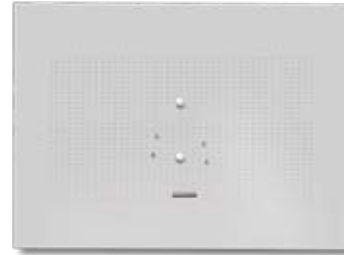
Lift pins and disappearing guides with camera well.
